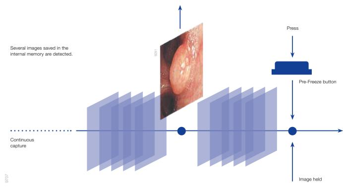
The system continuously buffers a series of images. When you take an image, it automatically analyzes the previous pictures and selects the sharpest one.
